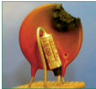
Figure 6b. MOV/TCO combination
