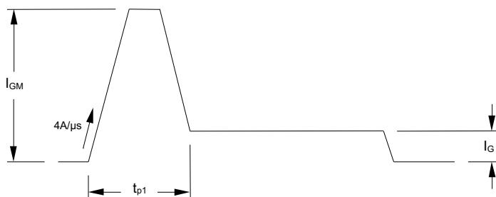
The magnitude of  $I_{GM}$  should be between five and ten times  $I_{GT}$ , which is shown on page 2. Its duration ( $t_{p1}$ ) should be 20 $\mu$ s or sufficient to allow the anode current to reach ten times  $I_L$ , whichever is greater. Otherwise, an increase in pulse current could be needed to supply the necessary charge to trigger. The 'back-porch' current  $I_G$  should remain flowing for the same duration as the anode current and have a magnitude in the order of 1.5 times  $I_{GT}$ .
