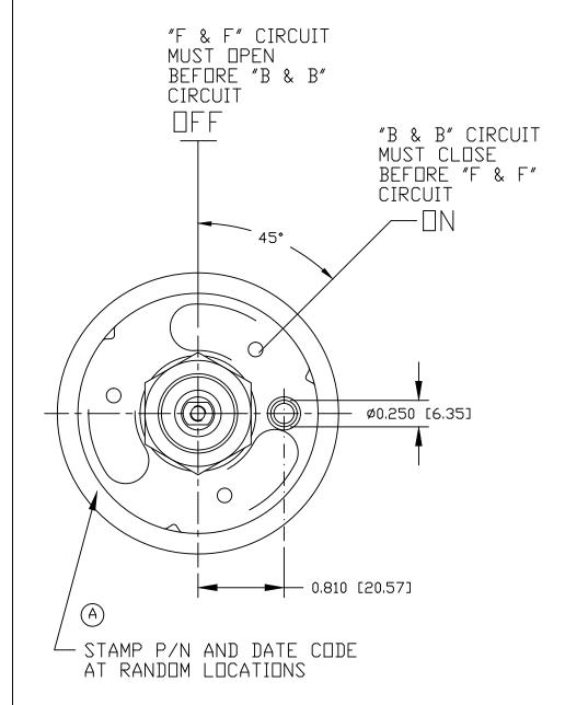
SCREW, #8-32 & LOCKWASHER – SHAFT -MOUNTING STEM, BRASS -HEX NUT, BRASS 2 HEX NUT, 3/4-16, - LOCKWASHER BRASS, PLATED — STUD, #10-32, BRASS, 2 PL — LOCKWASHER, 4 REQ'D - LOCKWASHER - CASE 0.775 [19.69] -G 0.800 [20.32] 3.470 [88.13]
