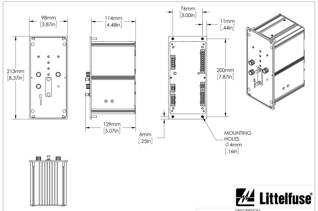
UNLESS NOTED OTHERWISE DIMENSIONS ARE IN INCHES TOLERANCES: TWO PLACE DECIMAL ±0.05 NOT DRAWN TO SCALE DESCRIPTION: NEUTRAL GROUNDING RESISTENCE MONITORING
