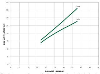
$\textbf{Note:} \ \text{Chart represents the range of Drop-Out, min to max, for a given Pull-in value of the MLRR-4 prior to modification inot the MLSM-4.}$
