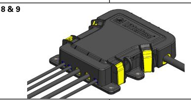
Replace the cover on the housing. Ensure that the cover seal is not being pinched or damaged.
