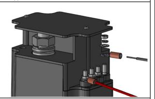
Strip all the wires that will be connected to the control coil and the contactor terminations with a wire stripper. Remove approximately ½ inch of the wire's insulation to expose the bare copper wire. Connect the control wires to the coil solenoid first, two outside terminal lugs. When installing the wires, be sure that a good electrical connection is made. Do not allow any loose strands to short against any equipment and cause electrical damage.
