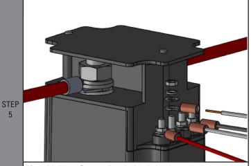
If an Auxiliary Contact is provided, connect the low power Line feed wire to one of the inner terminal lugs and the low power Load output wire to the remaining inner terminal lug. When installing the wires, be sure that a good electrical connection is made. Do not allow any loose strands to short against any equipment and cause electrical damage.
