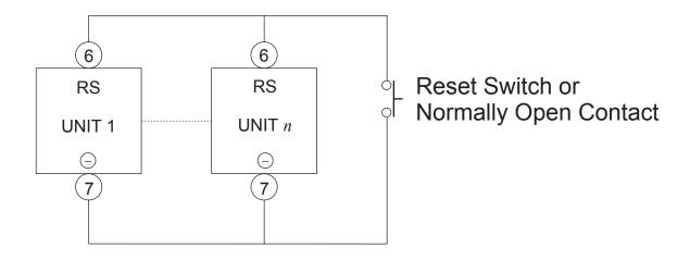
The equivalent circuit of the reset input is shown below.
