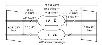
Coating Diameter (max): 0.5A-3.0A: 2.80mm 5.0A: 2.90mm
