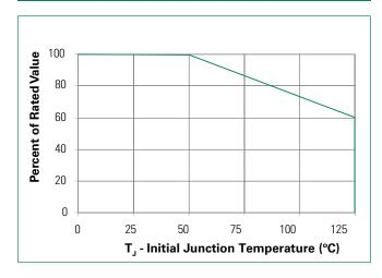
Figure 4 - Typical Peak Pulse Power Rating Curve
