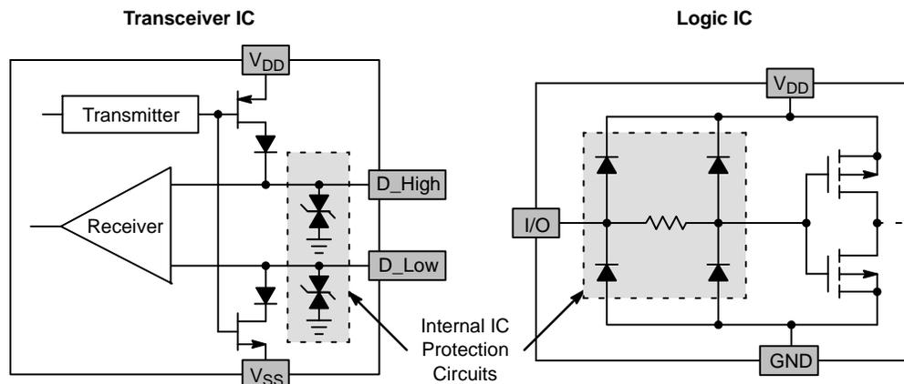
**Figure 1. Zener Diodes are a Popular Choice for the Internal Protection Circuit of a Transceiver IC that Requires Power Surge and ESD Protection. Diode Arrays are a Frequent Choice for the Internal ESD Protection Circuit of a Logic IC**
