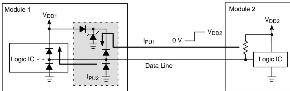
**Figure 11. Back Drive Protection can be Implemented by Adding an Avalanche and Blocking Diode to the Diode Array. The Blocking Diode Eliminates the  $I_{PU1}$  Current Path; However, Current Path  $I_{PU2}$  will Exist if the IC has a Diode Connected between the Output and Power Supply Pins**
