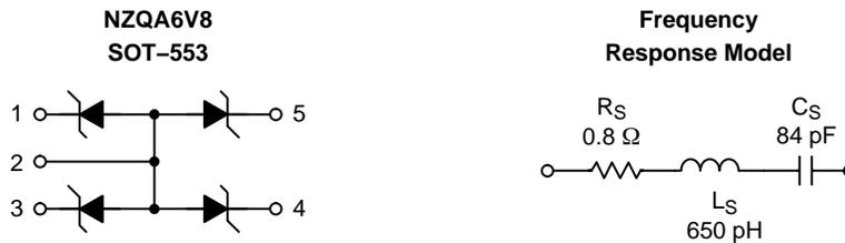
**Figure 14. The Frequency Response of an Avalanche TVS Diode can be Modeled by a Resistor, Inductor and Capacitance that are Connected in Series. This Model is Valid for Signals that are Smaller in Magnitude than the Clamping Voltage**
