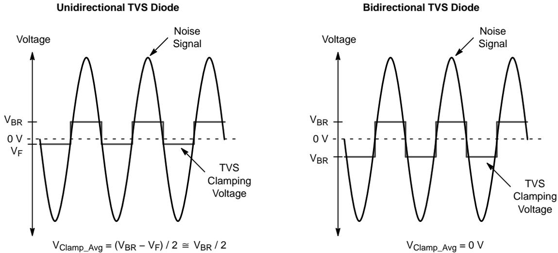
**Figure 12. The Average Clamping Voltage of a Unidirectional TVS Diode for a Sine Wave Input is  $V_{BR}/2$ . The Symmetrical Breakdown Voltages of a Bidirectional Device has an Average Clamping Voltage that is Biased at 0 V**
