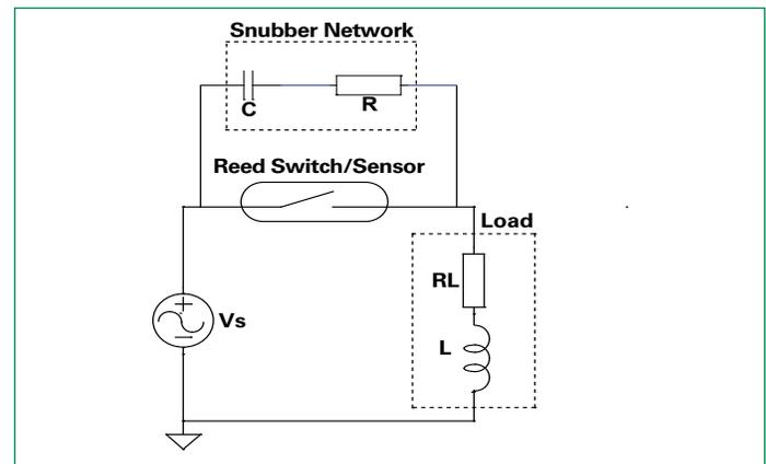
The values of the resistor and capacitor used in the snubber are by necessity compromises. The resistor value must be large enough to limit the capacitive discharge current when the switch contacts close, but small enough to adequately limit the voltage when the switch contacts open. Larger capacitor values decrease the voltage when the switch contacts open but they cost more and also increase the capacitive discharge energy when the switch contacts close.
