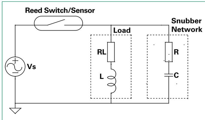
To select an approximate resistor value, use Ohm's law:  $V = I * R$ , or in this case  $R = V / I$ . Choose R between  $0.5 * V_{pk} / I_{sw}$  and  $3 * V_{pk} / I_{sw}$ , where  $V_{pk}$  is the AC peak voltage ( $V_{RMS} * 1.414$ ) and  $I_{sw}$  is the rated switching current of the reed switch or sensor. A lower R decreases the contact wear from arcing. A higher R decreases the contact wear from the capacitive inrush current.
