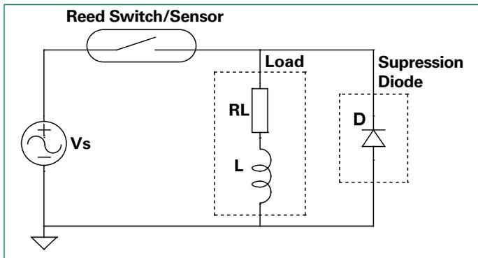
The MOV and TVS diode devices conduct current when a threshold voltage is exceeded. These devices are usually placed across (in parallel with) the switch contact. These devices can work well for lower voltages such as 24 VAC and can also work for higher inductance 120 VAC loads. MOV devices have more capacitance than TVS diodes. If an MOV is used, the effect of MOV capacitance should be reviewed. A separate Hamlin application note discusses capacitive loads.
