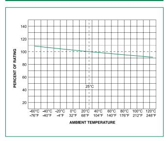
Note: Rerating depicted in this curve is in addition to the standard derating of 25% for continuous operation.
