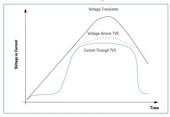
Figure 2: Peak Pulse Power Rating
