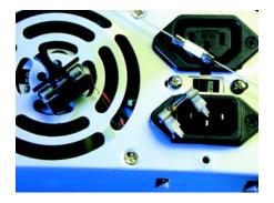
solder 5x20mm fuses when assembled with plug-on end caps. For these power supply types, there is a ongoing trend towards more compact form factors. TR5® and TE5® fuse types offer a PC board space savings of up to 65% when compared to traditional 5x20mm glass fuses. These fuse types are delivered in a taped format. They can be soldered directly to the PC board via auto-matic insertion equipment and offer lower
