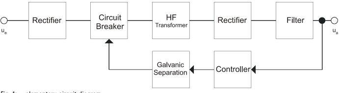
Fig. 1: elementary circuit diagram primary clocked switch controller
