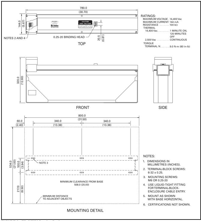
FIGURE 9. ER-25KV Sensing Resistor.
