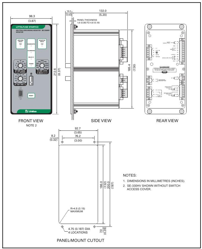
FIGURE 4. SE-330HV Outline and Panel-Mounting Details.
