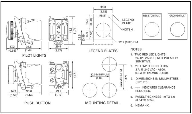
FIGURE 18. RK-332 Remote Indication and Reset.
