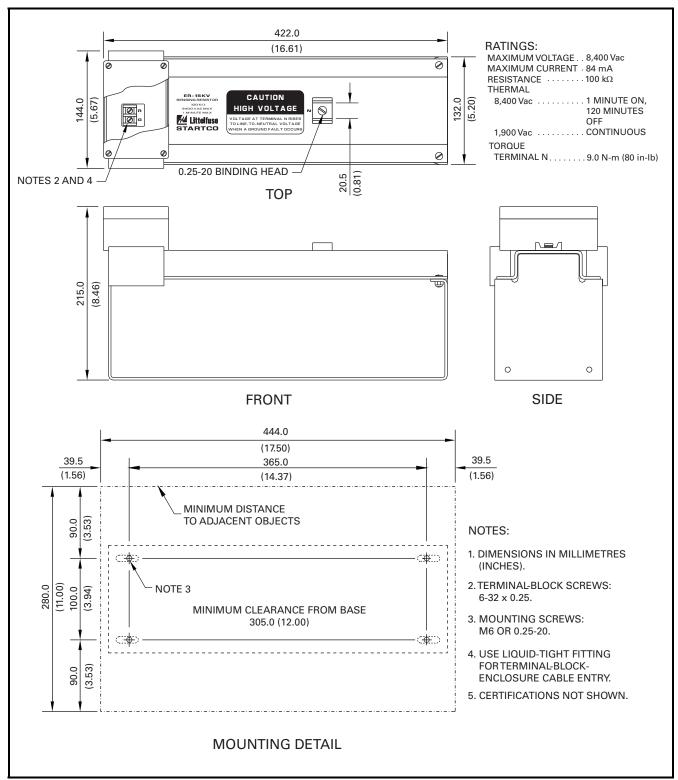
FIGURE 8. ER-15KV Sensing Resistor.
