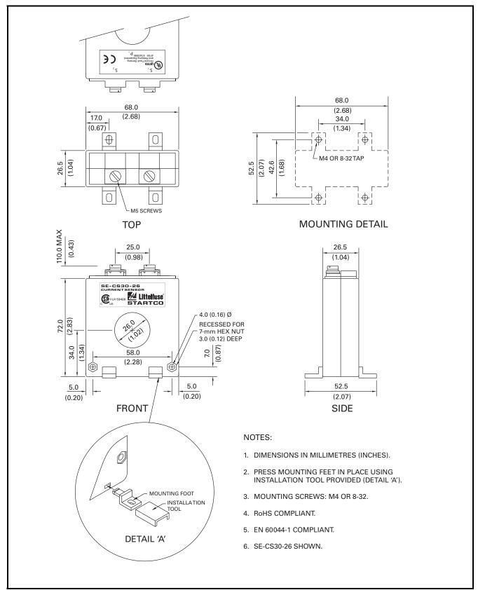
FIGURE 17. EFCT-26 and SE-CS30-26 Ground-Fault Current Sensors.
