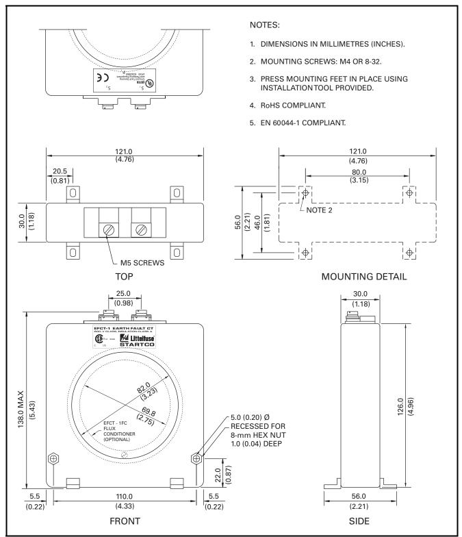
FIGURE 15. EFCT-1 Ground-Fault Current Sensor.
