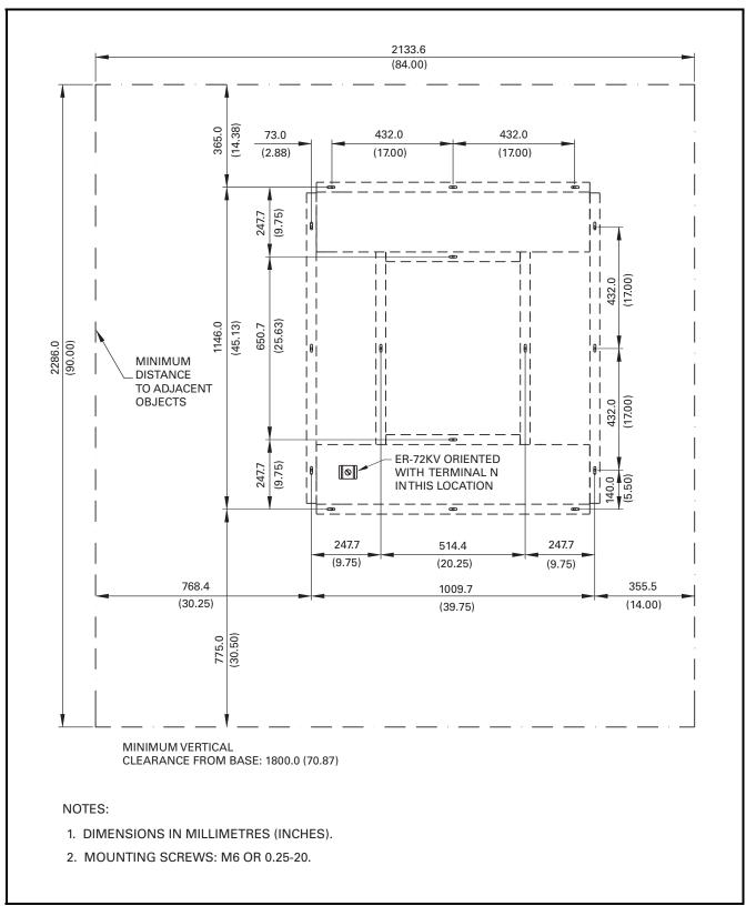
FIGURE 12. ER-72KV Sensing Resistor Mounting Details.
