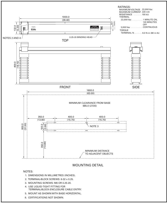
FIGURE 10. ER-35KV Sensing Resistor.
