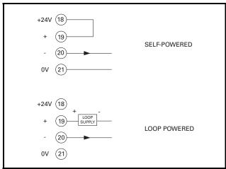
FIGURE 2. Analog-Output Connections.
