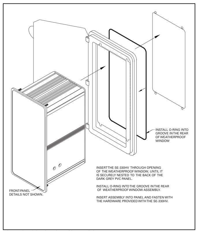
FIGURE 7. SE-IP65CVR-G Weatherproof Cover Installation.
