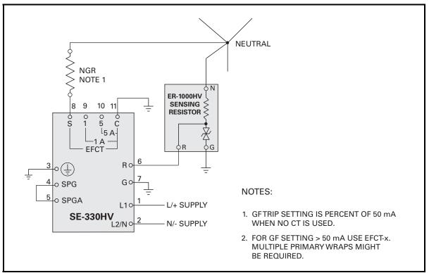
FIGURE 14. ER-1000HV Simplified Connection Diagram.
