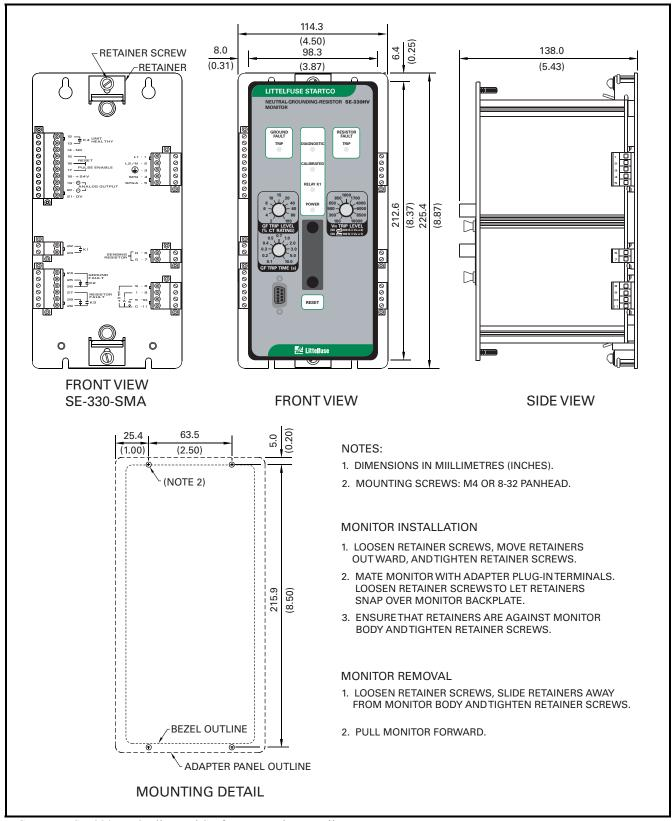
FIGURE 5. SE-330HV Outline and Surface-Mounting Details.
