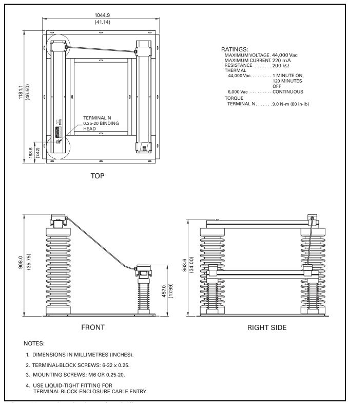
FIGURE 11. ER-72KV Sensing Resistor Outline.
