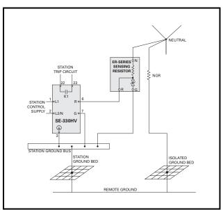
FIGURE 19. Simplified Isolated-Ground Connection.
