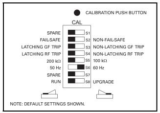
FIGURE 1. Configuration Switches.
