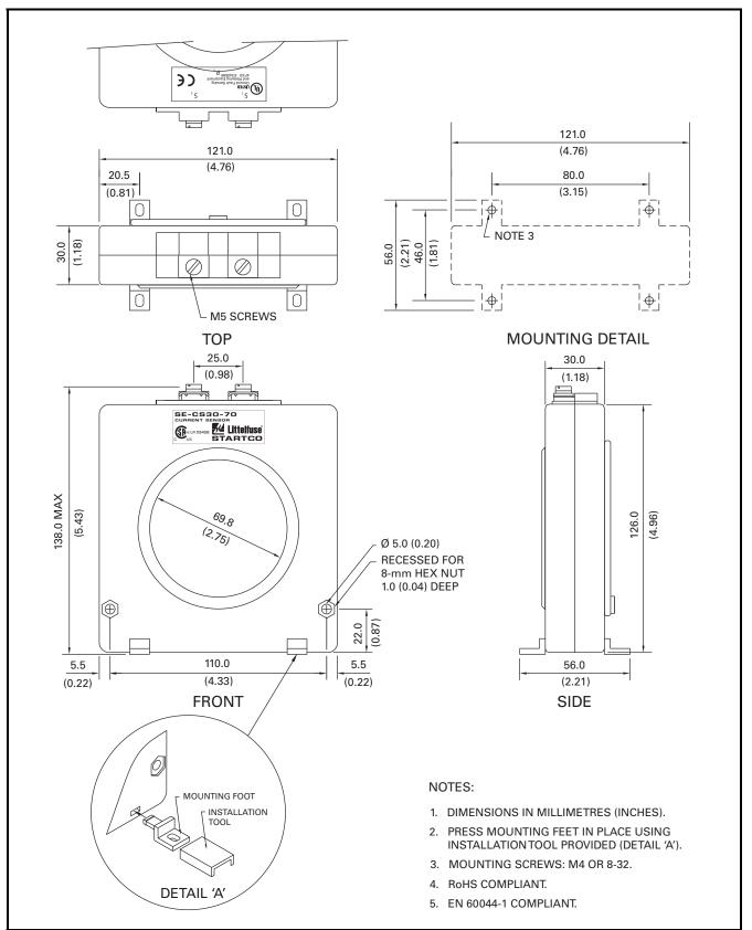
FIGURE 16. SE-CS30-70 Ground-Fault Current Sensor.
