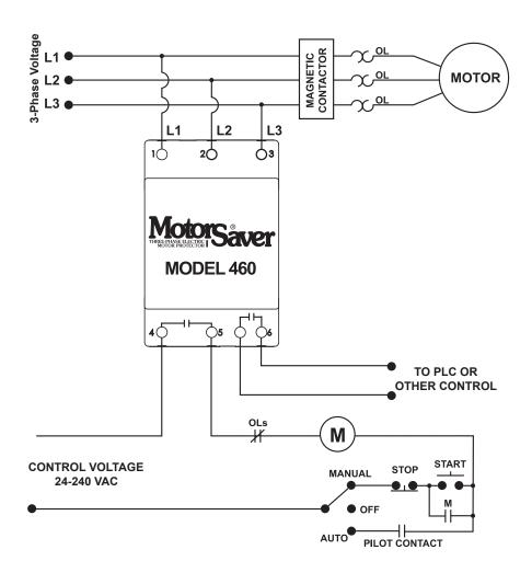
FIGURE NO. 1: CONTROL WIRING DIAGRAM
