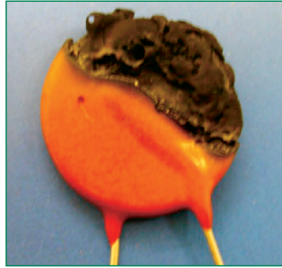
Figure 6a. Standard MOV
