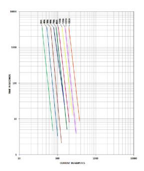
FI = 1.00 (max. operating current :  $1.0 \times I_{rat}$  at  $23^{\circ}$ C)
