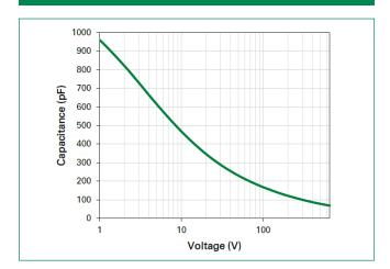
Figure 6: Capacitive Charge vs. Reverse Voltage
