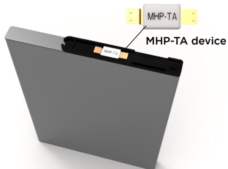
MHP-TA device connected to the positive terminal of a Li-Polymer cell
