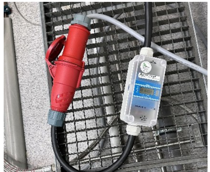
Figure 1: Eltako DSZ180CEE-32A MID 28032128 three-phase meter digital 10 A
