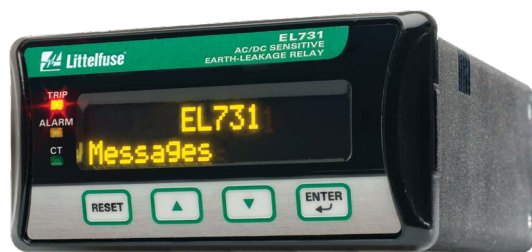
FIGURE 4: The EL731 is a sensitive ac-dc earth-leakage relay with programmable alarm and trip settings, relay, analog, and serial outputs, and a 32-character OLED display.
