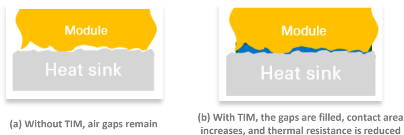
Figure 4. Improving Thermal Transfer by using Thermal Interface Material (TIM)
