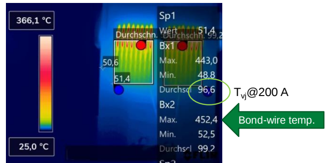
Fig. 5 Thermal image taken at 200 A per die
