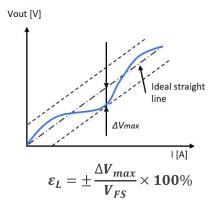
V<sub>FS</sub>: full scope output voltage
