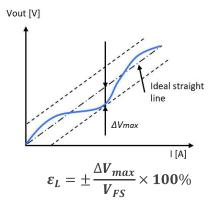
V<sub>FS</sub>: full scope output voltage
