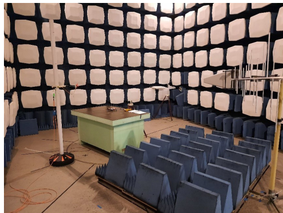
Figure 5. Radiated emission test chamber
