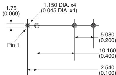
Note: Pin-to-pin tolerances are non-cumulative.
