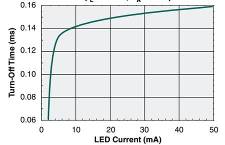
Typical I<sub>F</sub> for Switch Operation
