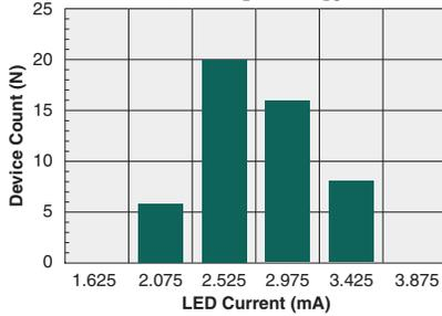
Typical  $I_F$  for Switch Dropout
