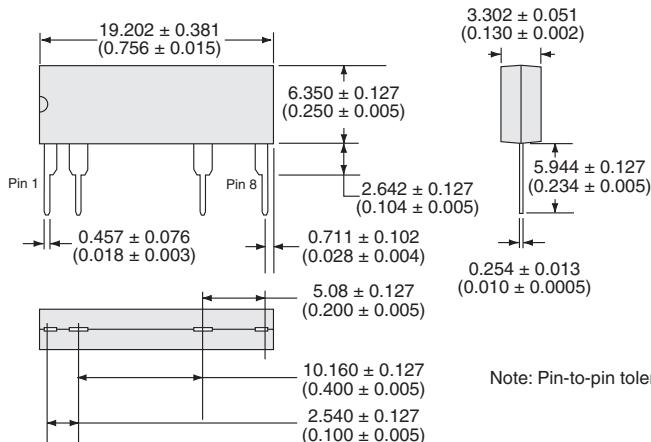
Note: Pin-to-pin tolerances are non-cumulative.
