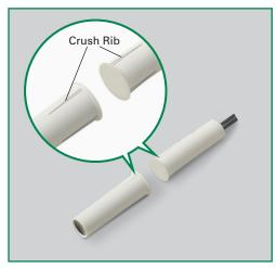
Three crush ribs, equally spaced on the outside diameter, compress when inserted into a mating hole.
