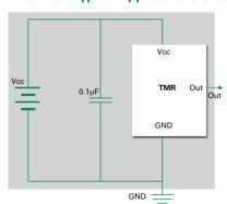
**Note:** It is strongly recommended that an external bypass capacitor be connected in-close-proximity to the device between the supply and ground pins to reduce noise. The recommended value for the external bypass capacitor is 0.1uf.
