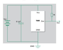
**Note:** It is strongly recommended that an external bypass capacitor be connected in-close-proximity to the device between the supply and ground pins to reduce noise. The recommended value for the external bypass capacitor is  $0.1\mu F$ .
