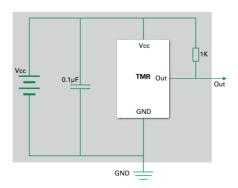
Note: It is strongly recommended that an external bypass capacitor be connected in-close-proximity to the device between the supply and ground pins to reduce noise. The recommended value for the external bypass capacitor is 0.1u.s.
