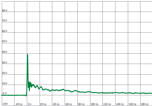
IEC 61000-4-2 +8 kV Contact ESD Clamping Voltage
