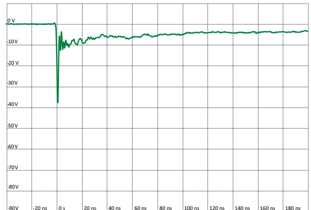
ISO10605 Contact Discharge Plot at -8 kV
