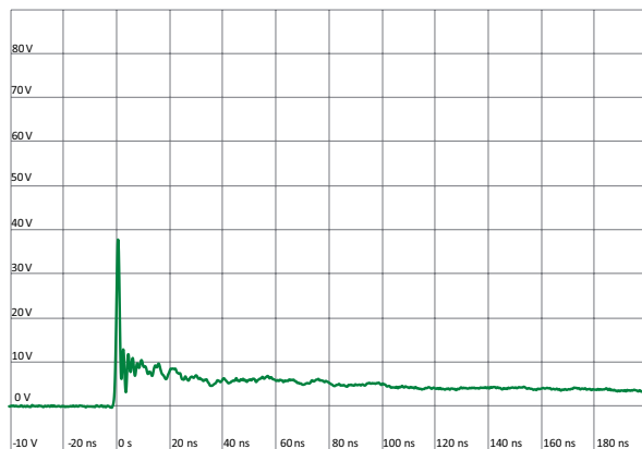
ISO10605 Contact Discharge Plot at +8 kV
