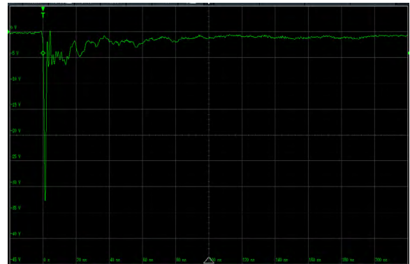
IEC 61000-4-2 -8 kV Contact ESD Clamping Voltage
