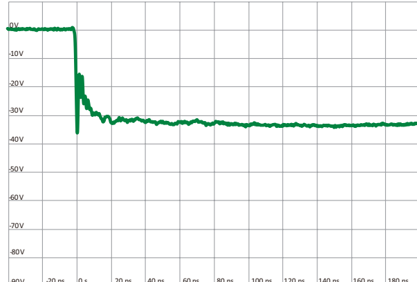
ISO10605 Contact Discharge Plot at -8 kV
