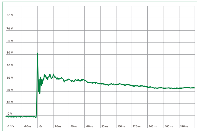
IEC 61000-4-2 +8 kV Contact ESD Clamping Voltage
