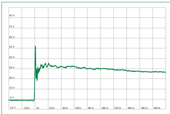
ISO10605 Contact Discharge Plot at +8 kV
