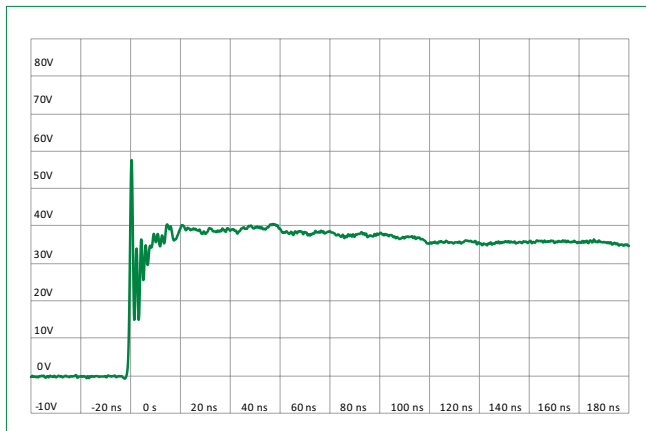
IEC 61000-4-2 +8 kV Contact ESD Clamping Voltage
