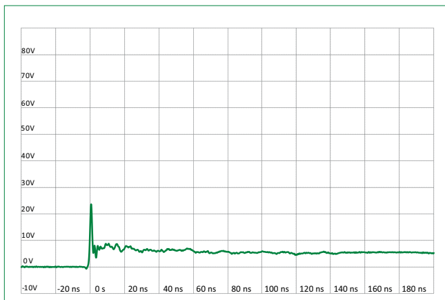
IEC 61000-4-2 +8 kV Contact ESD Clamping Voltage
