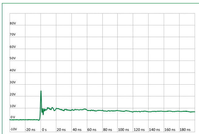
ISO10605 Contact Discharge Plot at +8 kV
