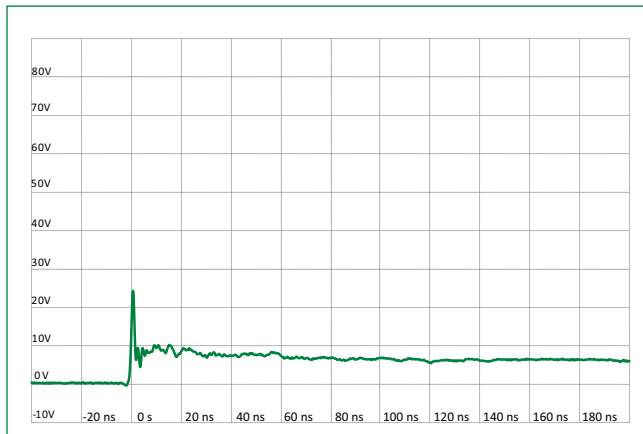
IEC 61000-4-2 +8 kV Contact ESD Clamping Voltage
