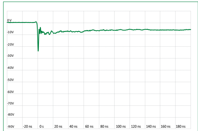
IEC 61000-4-2 -8 kV Contact ESD Clamping Voltage
