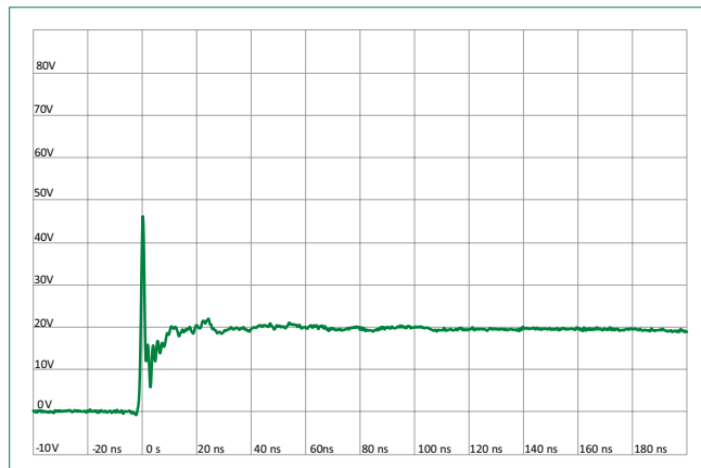
IEC 61000-4-2 +8 kV Contact ESD Clamping Voltage
