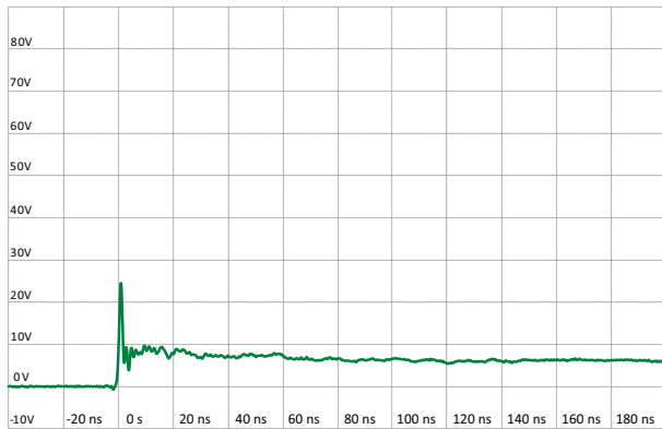
IEC 61000-4-2 +8 kV Contact ESD Clamping Voltage
