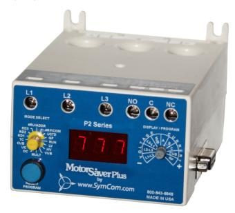
How to set the response to an underload can vary with circumstances. Take, for example, a lift station pump that takes in a rag, causing a small overload or underload. It may be worthwhile to set the protective relay to shut down for several minutes, and then make one restart attempt, allowing the debris an opportunity to free itself. If the problem returns then the relay should shut off the motor, alarm, and require manual intervention.
