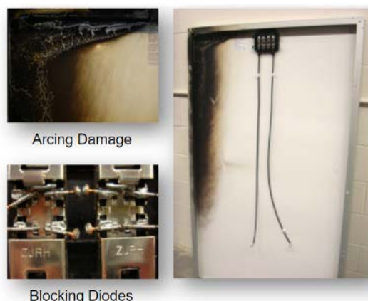
FIGURE 5. Mono-silicon panel failures include arcing, burning and diode destruction.
