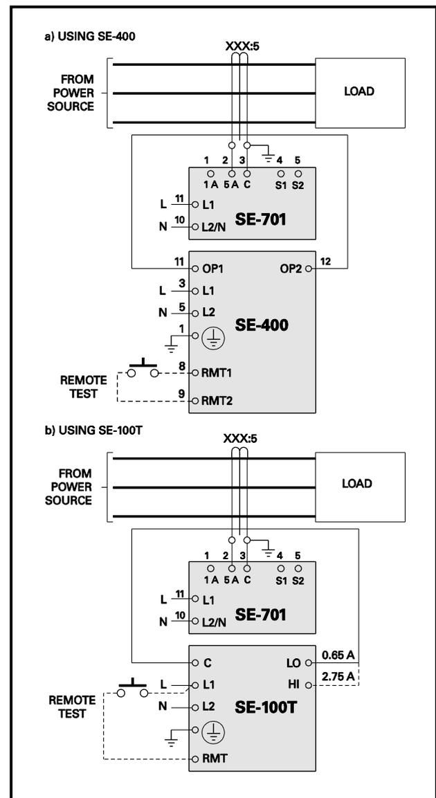
FIGURE 11. Ground-Fault-Test Circuits.
