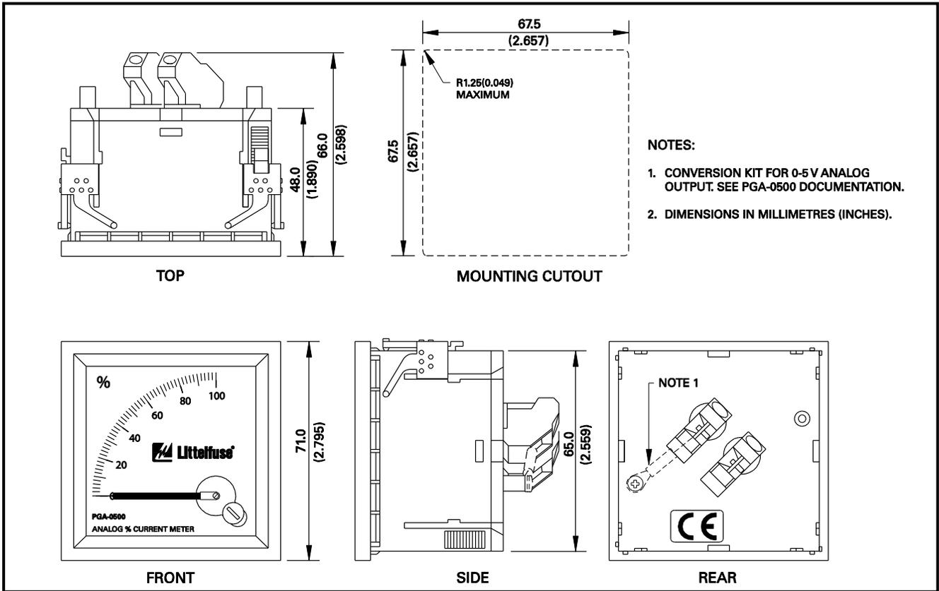
FIGURE 10. PGA-0500 Analog Percent Current Meter.
