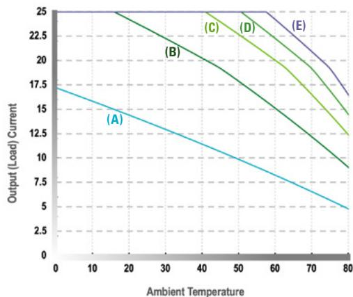
(A) 6 °C/W: Heatsink (C) 2.1 °C/W: Heatsink (E) 1.5 °C/W: Heatsink
