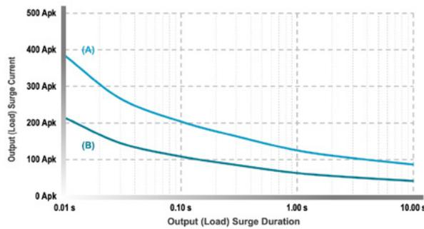
**(A) Single Pulse Surge:** Initial SSR internal temperature at 25°C (cooler state from minimal or no operation).
