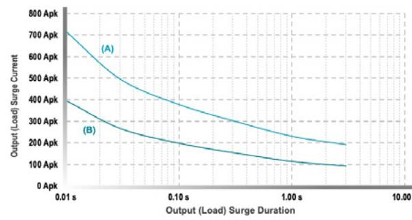
**(A) Single Pulse Surge:** Initial SSR internal temperature at 25°C (cooler state from minimal or no operation).
