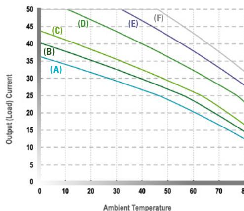
(A) 2.1 °C/W: Heatsink (C) 1.5 °C/W: Heatsink (E) 0.7 °C/W: Heatsink
