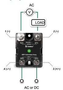
The diagram shows the correct configuration for connecting the solid-state relay to either an AC or DC power source. The relay has four terminals:
